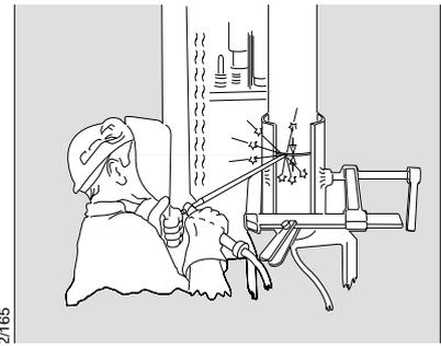
inclusions or pores, and no embrittlement either in the weld itself or in the zones affected by the heat of the weld.
