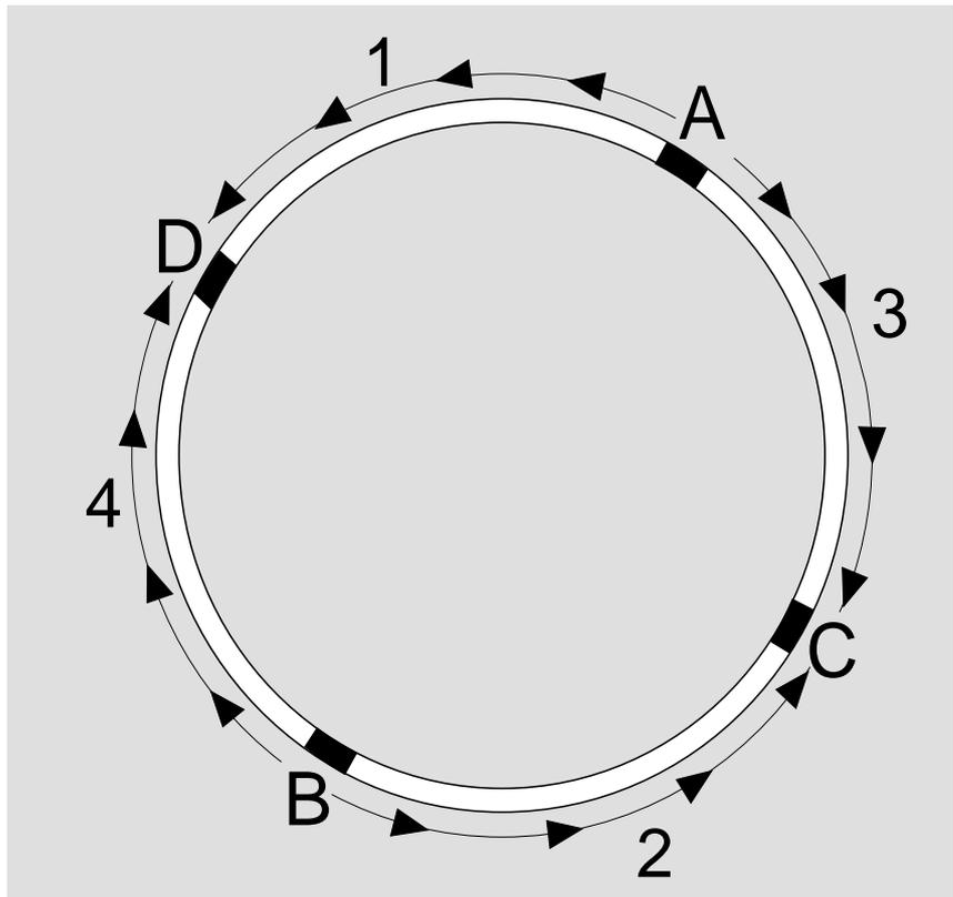
electrodes with a diameter of 2.5 mm, at approx. 85 A. Leave a 2 mm gap between the casing tubes to facilitate welding. The welding sequence is shown below.
