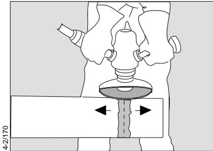
hole wall as the tubes are driven down. Use the same grinding machine as for bevelling. Grind only along the longitudinal axis of the tube. Scratches caused by grinding across the longitudinal axis of the tube can cause increased tension in the joint. Grind until the surface across the welded joint is flat.
