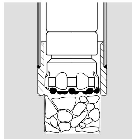
**N.B.** The guide sleeve used in TUBEX XL drilling must be removed from the top sub of the DTH hammer before normal drilling can continue. This is because its outside diameter is greater than the inside diameter of the casing shoe.
