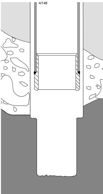
With the TUBEX XL equipment removed, it is possible to continue drilling the hole through the bedrock, using conventional drilling equipment. To prevent the ingress of surface water, e.g. in water-well drilling, the casing tubes can be grouted into position where they meet the bedrock. In any event, they should be driven firmly down to the actual bottom of the reamed hole.
