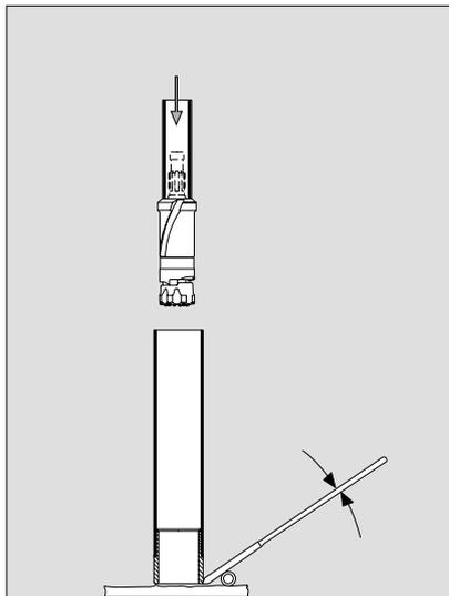
the percussion mechanism of the DTH hammer be used to get the TUBEX XL equipment through the casing shoe! At worst, this could result in the equipment jamming inside the casing shoe, which would then have to be cut open in order to remove the TUBEX XL equipment.
