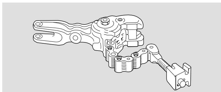
If the drill rig is intended for larger TUBEX XL equipment, it will probably be equipped with a hydraulic breakout table and an adjustable chain tongue. The equipment will make all breakout operations easier.
