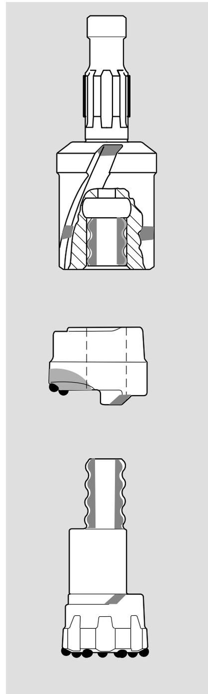
Different components in the TUBEX XL package have different service lives. A rough rule of thumb is that two reamers are used to one pilot bit, and two pilot bits are used to one guide device.
